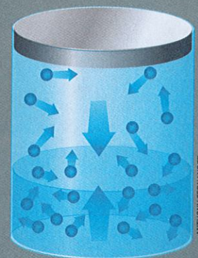
Figure 1. Vapor pressure is a measure of the force exerted by a gas above a liquid in a sealed container.
